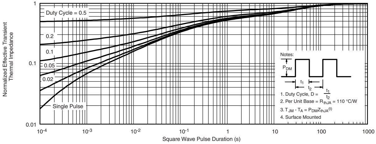
Normalized Thermal Transient Impedance, Junction-to-Ambient
